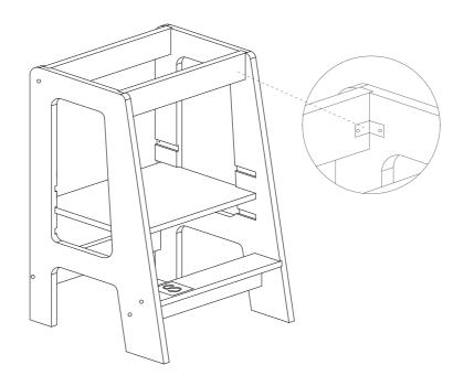
\*\*L-Brackets and covers RECOMMENDED to be installed- drill is required\*\*
